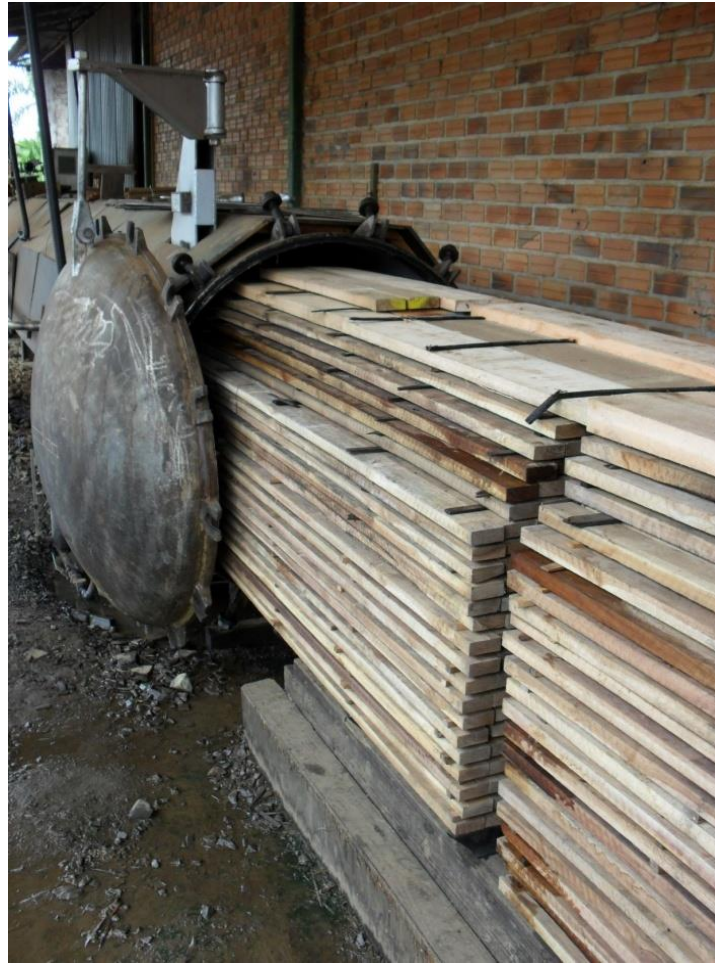
Figure 2: Example of wood being loaded into the equipment.
